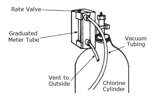
**NOTE:** Vent tubing should always be connected and run to a safe location (outside of any building). A vent bug cap (provided with every Archer Instruments vacuum regulator) should be fitted over the end of vent tubing to prevent insects from entering the equipment.
